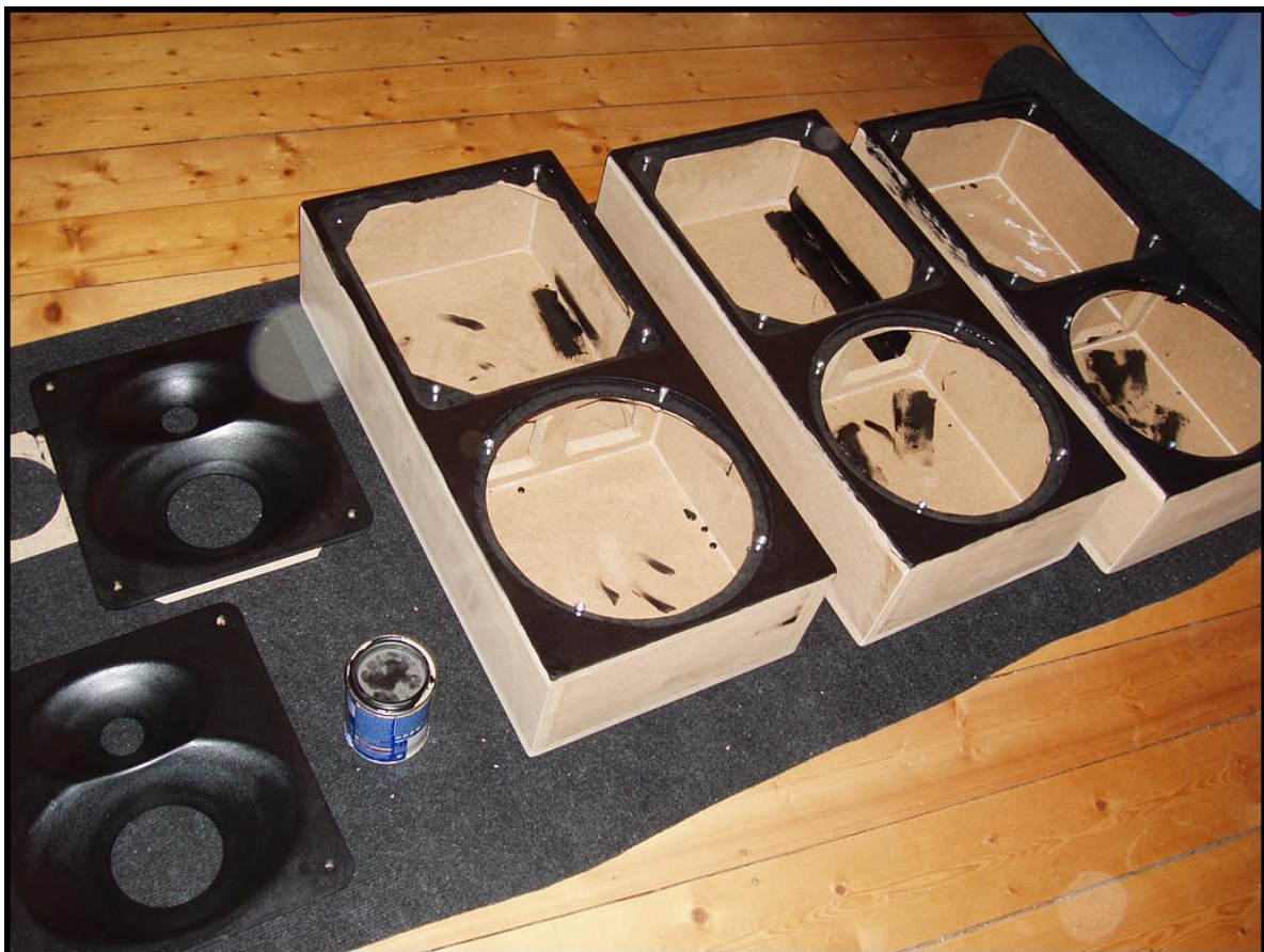
Figure 4- Painting of the enclosure parts
