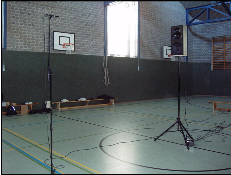
Figure 13: Measuring arrangement with measuring distance of 3 m
