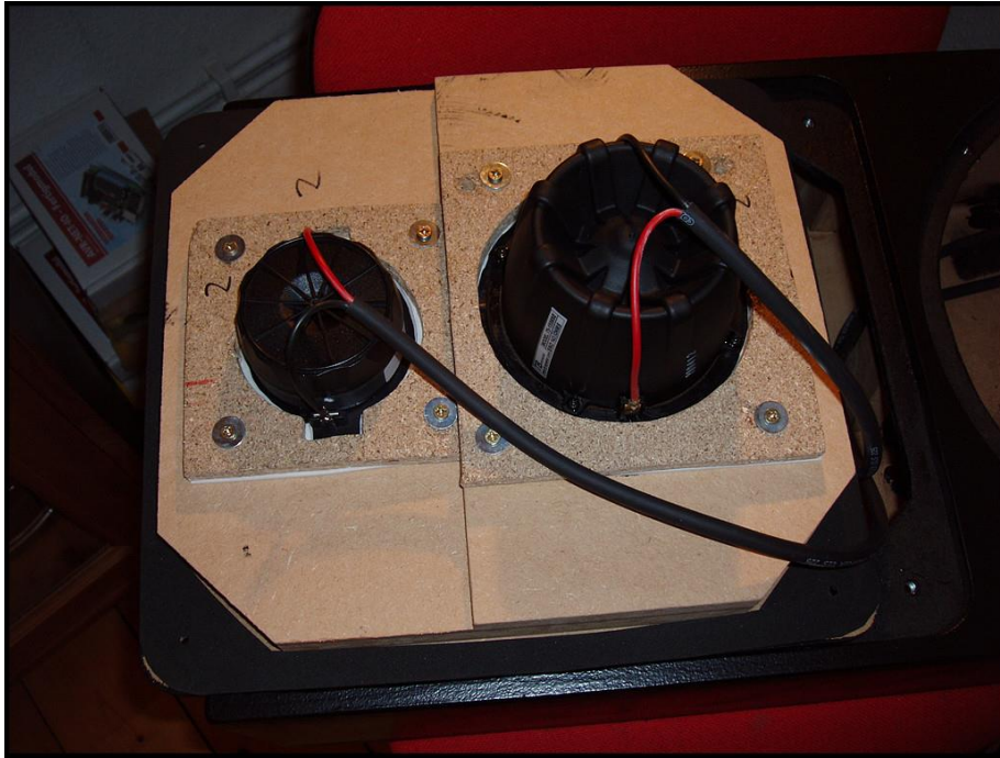
Figure 5: Mount the drivers on the waveguide
