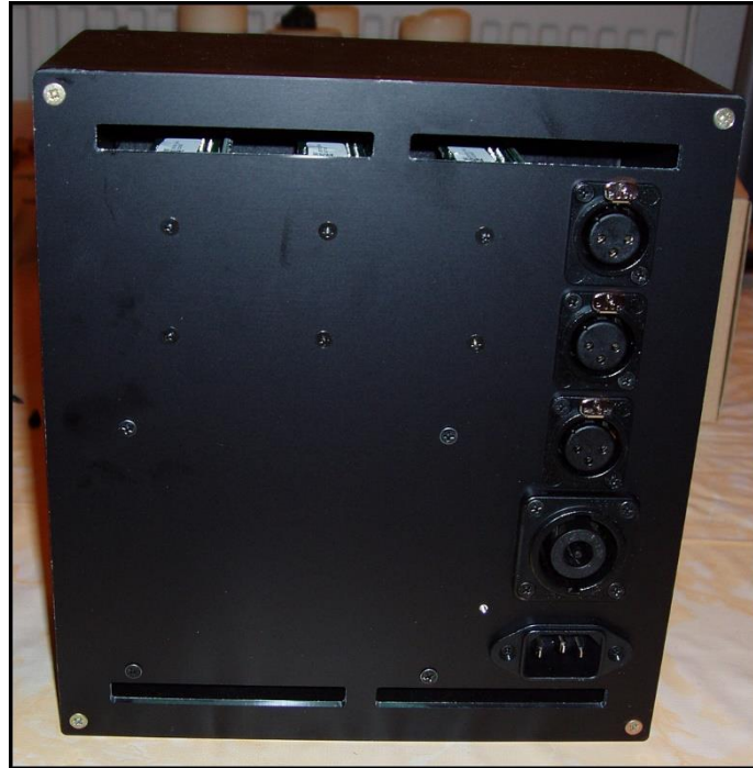
Figure 11: Fully assembled power amplifier housing
