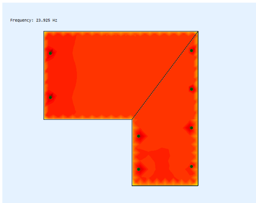
Figure 5: 1. Longitudinal mode (approx. 24 Hz) throughout the room
