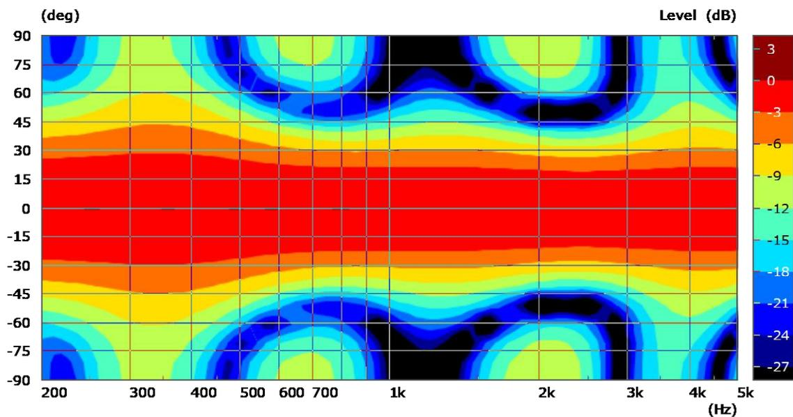
Figure 7: Directivity with linear-phase filters
