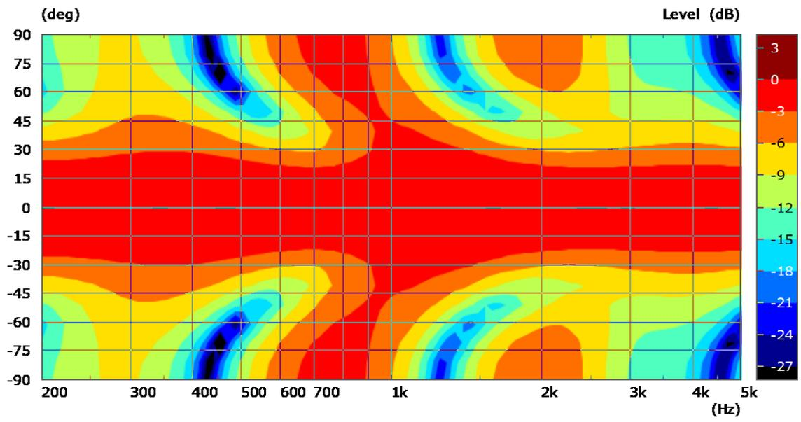
Figure 8: Directivity with minimum-phase filters
