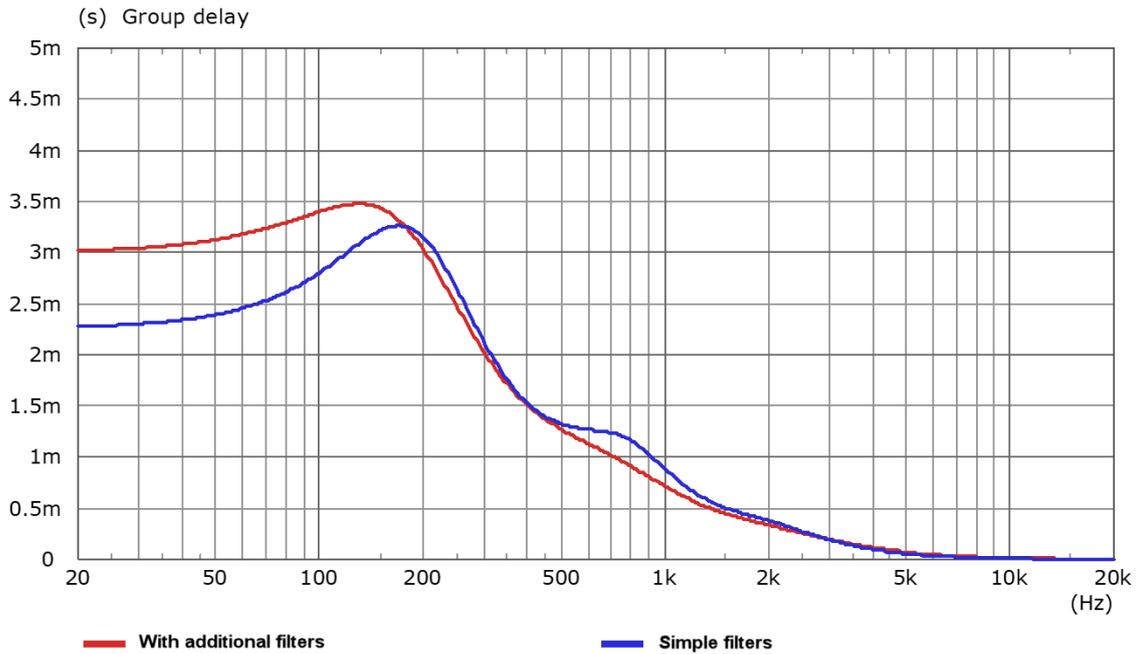
Figure 10: Group delay distortion
