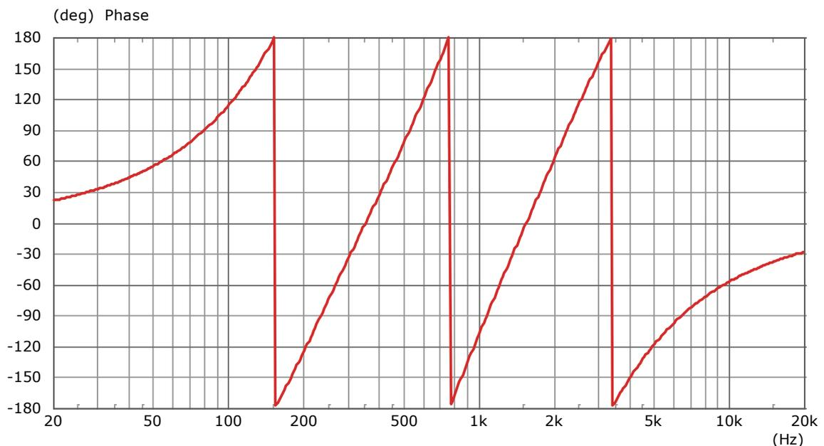
Illustration 11: FIR correction filter for the overall phase response
