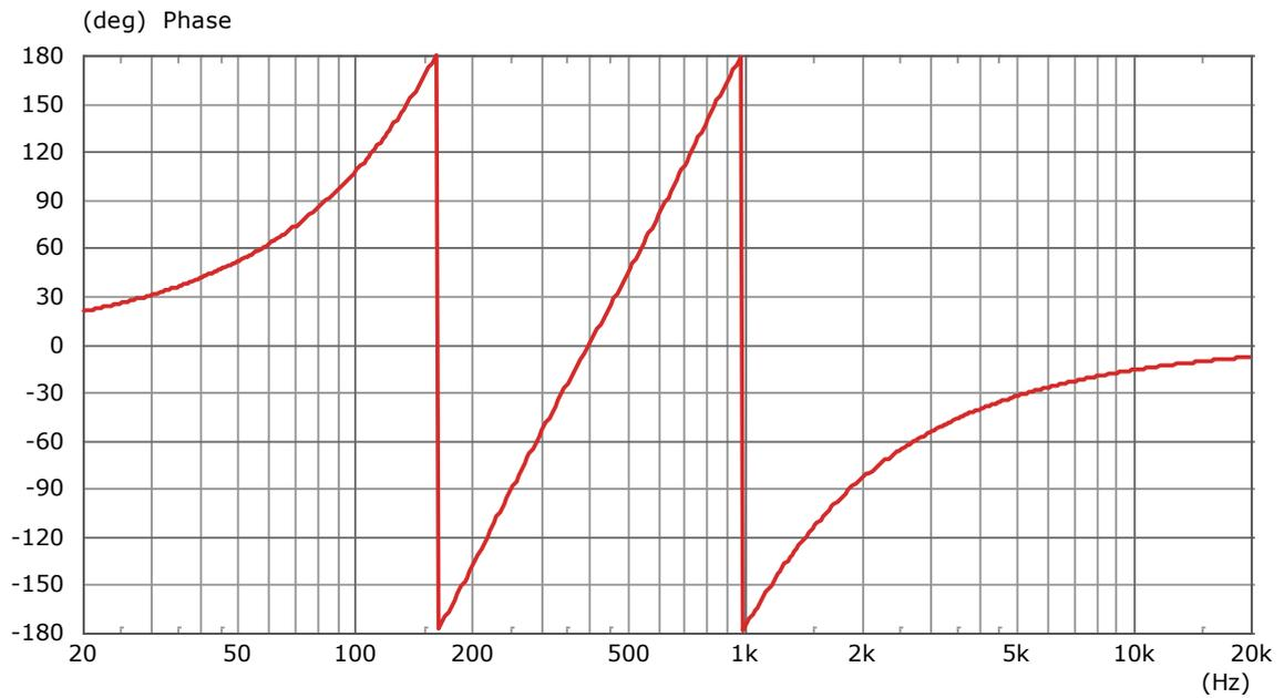
**Illustration 14: FIR compensation filter for phase distortion of IIR filter**
