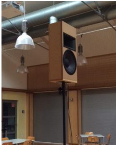
Illustration 48: 2-Way Speaker with Horn
