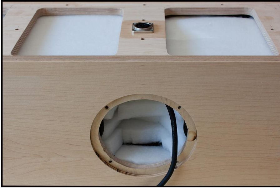
Figure 18: Filling with Iso Bond WLG 045
