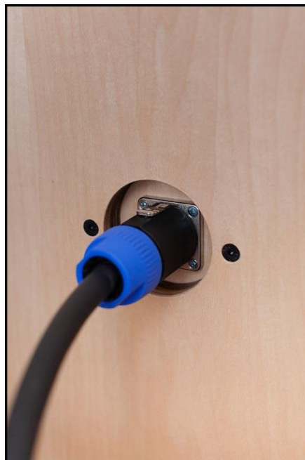
Figure 17: Rear panel with speakOn jack
